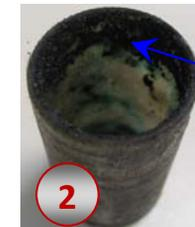
Spatter build up in nozzle insulator. Beginning of insulating material breakdown
