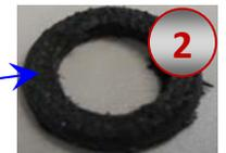
Insulating washer beginning to breakdown.
