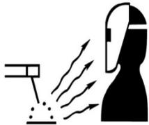
**WARNING – A WELDING ARC EMITS ULTRAVIOLET (UV) AND OTHER RADIATION AND CAN CAUSE SERIOUS INJURY TO UNPROTECTED SKIN AND EYES.**
