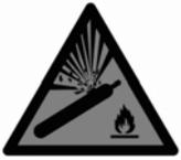
**WARNING – Compressed gas cylinders contain gas under high pressure and/or flammable gas. If damaged, the cylinder can explode.**
